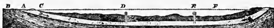
FIG. 37.—Ideal section illustrating the chief requisite conditions of artesian wells. A , a porous stratum; B C , impervious beds below and above A , acting as confining strata; F , the height of the water level in the porous bed A , or, in other words, the height of the reservoir or fountain head; D E , flowing wells springing from the porous water-filled bed A .—After CHAMBERLIN.
